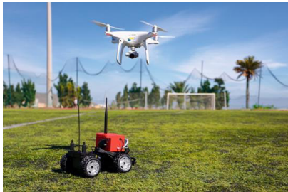
Fig 11: Prototype for the autonomous GPS tracking system, with the drone following a remote control vehicle.
