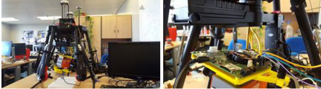
Fig 2: On the left, the Dji Matrice 600 in the laboratories with the RONIN-MX gimbal and the hyperspectral Specim FX10. On the right, a detail of the NVIDIA Jetson TK1 GPI on top of the camera.
