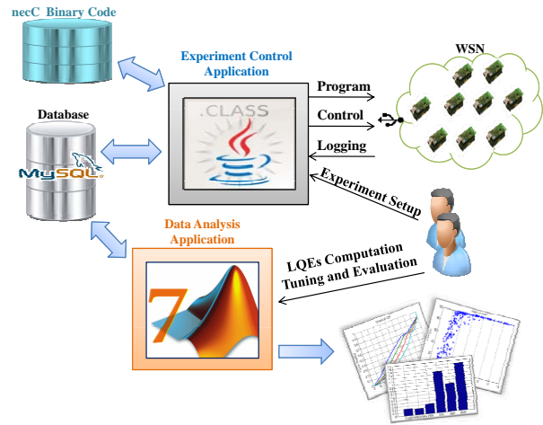
Fig. 2. RadiaLE software components
