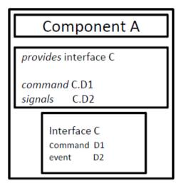
A TinyOS component providing an interface
