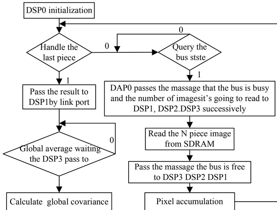
Fig. 5. The flow chart of the bus arbitration mechanism used in this paper.
