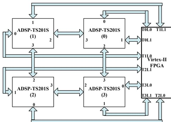
Fig. 2. Framework of the Link port connections inside a DSP cluster.
