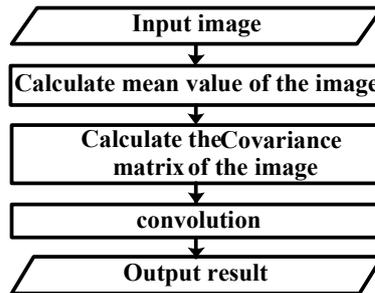
Fig. 3. RX anomaly detection algorithm based on a single DSP.
