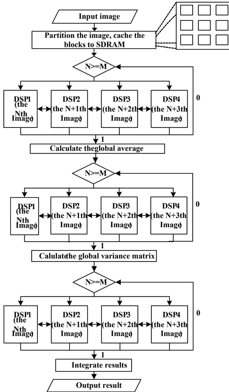
Fig. 4. RX anomaly detection parallel procedure based on 4-DSP.
