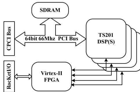
Fig. 1. Framework of the system bus connection.
