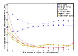
Figure 6: The impact of the number of the dispatchers on the protocol delay
