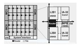
Figure 1: Intel's Single-Chip-Cloud (SCC)
