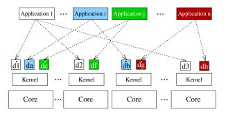
Figure 2: Architectural structure of the assumed model
