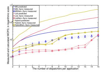
Figure 7: The impact of the number of the dispatchers on the protocol delay
