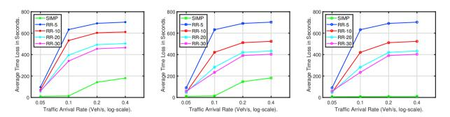
Fig. 2: Average Time Loss results in seconds, for **Scenarios-1**, **2**, and **3** with 30Km/h speed limit from left to right.
