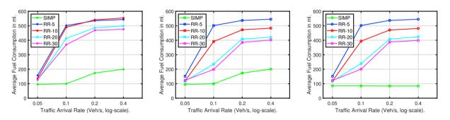
Fig. 5: Average Fuel Consumption results in ml, for Scenarios-1, 2, and 3 with 50Km/h speed limit from left to right accordingly.
