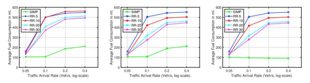
Fig. 3: Average Fuel Consumption results in ml for Scenarios-1, 2, and 3 with 30Km/h speed limit from left to right.
