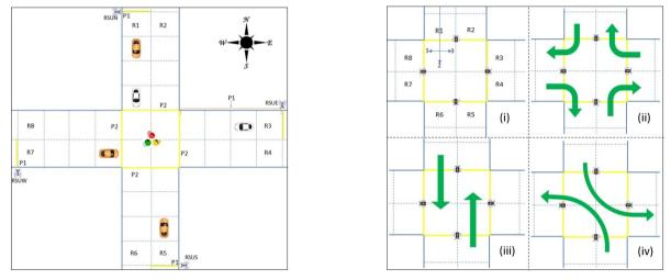
(a) IIMA on a four-way single-lane intersection (b) Direction codes and examples of crossing maneuvers Fig. 1: Intelligent Intersection Management Architecture (IIMA); Direction codes: 1-right, 2-straight, 3-left; and Crossing maneuvers: (ii) Right-crossing; (iii) Straight-crossing; and (iv) Left-crossing.
