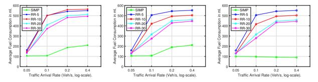
Fig. 3: Average Fuel Consumption results in *ml* for Scenarios-1, 2, and 3 with 30Km/h speed limit from left to right.
