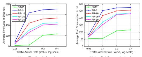
(a) Avg. Time Loss in Seconds. (b) Avg. Fuel Consumption in ml. Fig. 6: Time Loss and Fuel Consumption results for Scenario-4 with 30Km/h speed limit.
