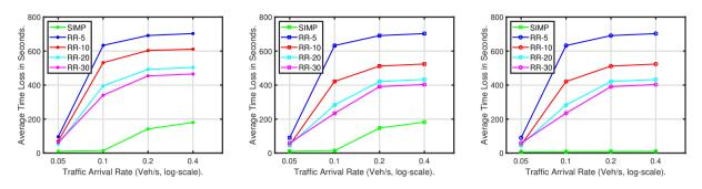
Fig. 2: Average Time Loss results in seconds, for Scenarios-1, 2, and 3 with 30Km/h speed limit from left to right.
