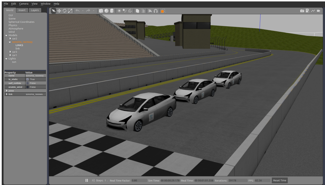
Figure 3.5: Simulation with three independent controlled Prius vehicles in the same Gazebo simulation.
