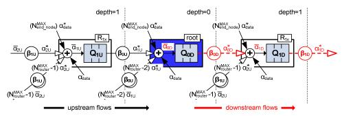
Figure 2. The queuing system model for upstream and downstream flows.
