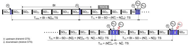
Figure 5. The worst-case service latencies for a flow along the longest path in the WSN related to the example in Figure 1.
