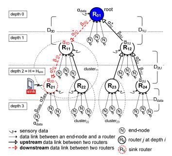
Figure 1. The cluster-tree topology and data-flow models.
