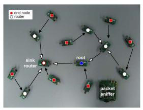
Figure 6. The test-bed deployment for  $H_{sink} = 1$ .
