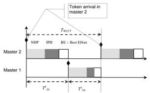
Fig. 2 Traffic allocation example for a 2-master network
