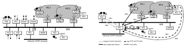
Fig. 3. RFieldbus network topology (left), Multimedia streams (right)
