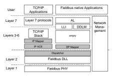
Fig. 1. PROFIBUS and TCP/IP integration
