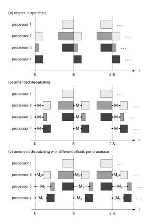
Figure 9: Example of dispatching, in (b) and (c), with x-reserves offset by  $M < 2 \cdot \alpha \cdot S$  time units, vs the original dispatcher (a). Reserves of different split tasks are colored differently.
