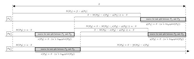
Figure 3: A detailed view of a timeslot, the reserves and their durations, used by our dispatching algorithm that is suited for implementation. The reserves for the split task shared by  $P_1$  and  $P_2$  and shared by  $P_2$  and  $P_3$  are shown by rectangles.
