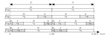
Figure 4: Execution timeline showing how tasks execute if all tasks arrive at time 0.
