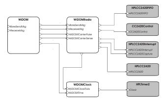
Figure 2. TinyOS component assembly.
