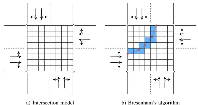
Fig. 1: Intersection modeled as a matrix of reservation tiles
