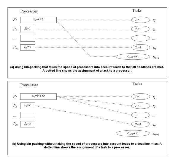
Figure 1. It is important to exploit knowledge of the speed of the processors when assigning tasks to processors. Otherwise, the speed competitive ratio can approach infinity.
