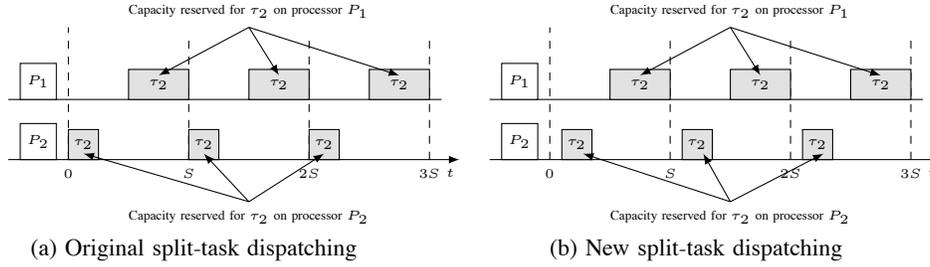
Figure 2. An example of the operation of slot-based task-splitting multiprocessor scheduling. Task  $\tau$  is a split-task. A non-split task executes only on its dedicated processor; it can execute in a reserve but it does so with a lower priority than a split task.
