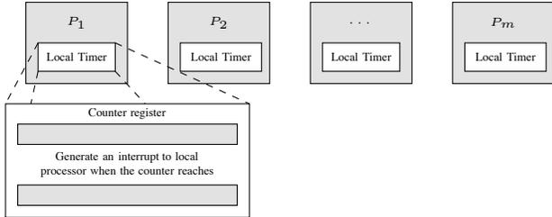
Figure 1. Each processor ( $P_i$ ) has a local timer.
