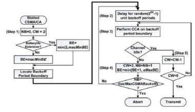
Figure 2. The IEEE802.15.4 Slotted CSMA/CA Algorithm
