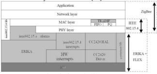
Figure 4. System Architecture
